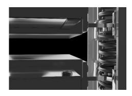
When pressing in a stack, each plate gap has to close together simultaneously so that all levels experience the same pressure at the same time. Strong spring force separation between plates makes this possible. 4 precision linear guides along with these springs also help to keep your plates even and resist tilting while pressing.
