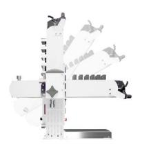
When rosin is pressed on horizonal plates, oil tends to puddle inside the folded parchment paper before it is expelled out of an opening. Our press body rotates up to 90 degrees allowing gravity to help oil escape through downward facing openings quicker. Falling oils then hit the surface below and flatten out into a puddle. Vertical heat plates along with an optional cooled catch surface all help to cool fresh pressed oil quicker, preserving its profile as much as possible.
